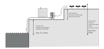
At shallow heads (1m), the Futurepump SEI can deliver up to 0.44 litres per second, which is 1,600 litres per hour or over 9,500 litres per 6-hour pumping day.
