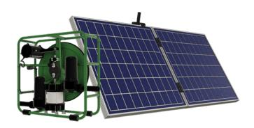
Futurepump solar pumps have three main parts: the power source (**PV panels**) which convert sunlight into electrical energy to drive, the **DC motor** that turns a flywheel which drives a reciprocating, positive displacement, high efficiency **piston pump**.
