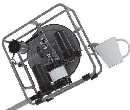
EN Fill the pump chamber with water.
