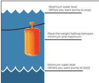
Example of float switch in 'tank full' position. Pump is turned off.
