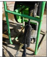
Step 2: Slide the weight along the wire so when installed it will hang halfway between the minimum and maximum water levels.
